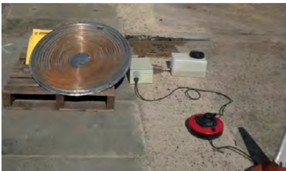
Figure 2: Solar photo-reactor detoxifying river water in Operation at University of Greenwich, Medway Campus, Kent, UK.
